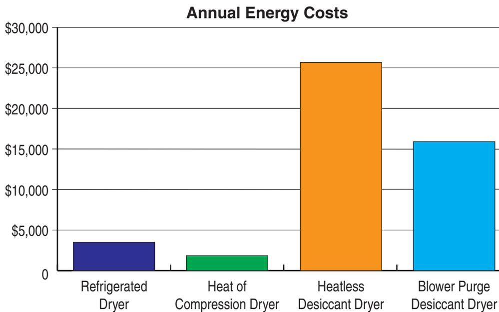
*Based on 8760 hours of operation, maximum ambient temperature 100°F, air pressure at dryer inlet 100 psig, maximum air temperature at dryer inlet 100°F, maximum air flow rate of 1000 scfm, and \$0.10/kWh.*
